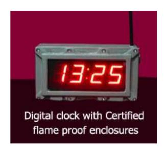
Each FLP Clock includes a 433 MHz transceiver. The FLP clocks receive the data from the master clock and update the accurate time. They are enclosed in a Certified Flame Proof Enclosure. These clocks can cover large areas indoors (up to 500 meter radius. The clocks incorporate frequency hopping / spread spectrum (FH/SS) technology coupled with DES data encryption to be sure no one tampers with time transmissions, and are free from interference.
